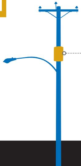
**Small Cell:** Small cell technology is much more discreet, mounted on existing structures like rooftops and utility poles. Sometimes, they are accompanied by refrigerator-sized equipment. Because small cells only supply a few hundred feet of coverage, they are best suited for dense areas like downtowns.
